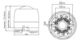
G(10), D1(9), D2(7): Connecting with 24VDC power, polarity-sensitive. G connects with positive output, D1 with positive input and D2 with negative.
