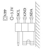
2. Tone 2: Jumper should be inserted in two pins on the other side as shown below.
