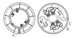
The sounder base does not require cabling. It will share the termination of the detector
