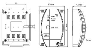
The detector and the gas stove should be placed in the same room. The detector should be mounted within 30cm -60cm to the floor. The detector should be within 1.5m -4m to the gas resource or the gas stove.
